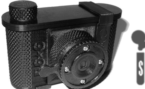
The P6\*6 is assembled from 3D printed parts, and is glued and fastened together with 3mm nuts and bolts. All individual parts print without support and fit on a six-inch square print bed.
