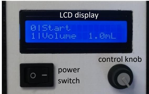
*User interface of the pump: The menu item "0|Start" is currently selected - pushing the control knob now would initiate pumping.*
