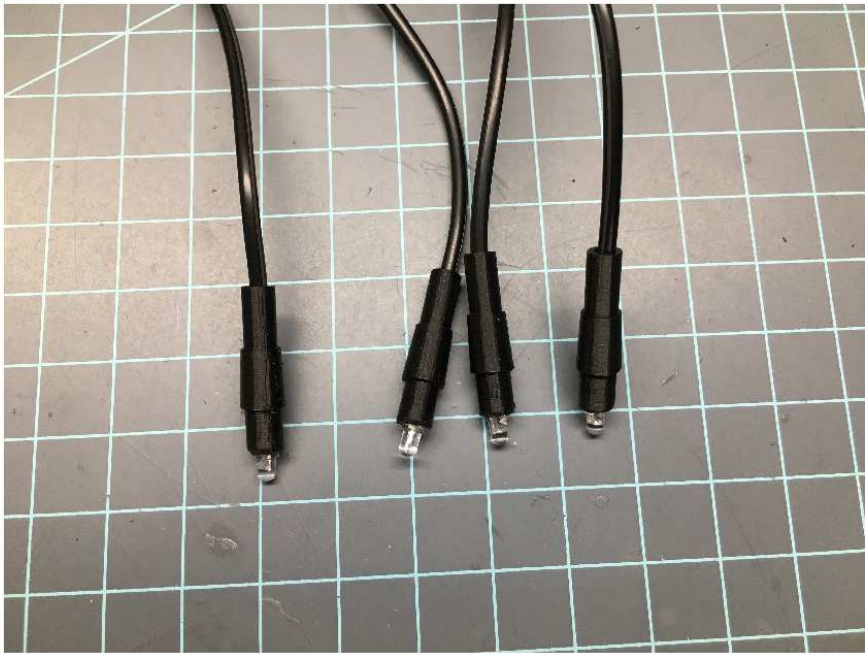
Glue base of LED to spark plug boot.
