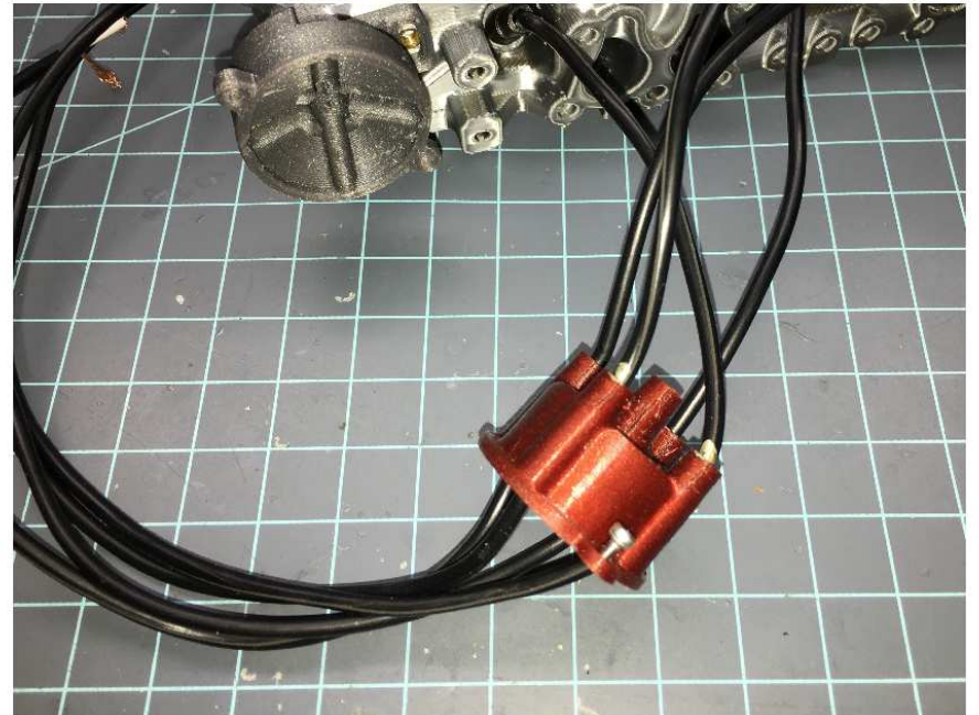
Mark coaxial wire where it goes into the distributor cap.
