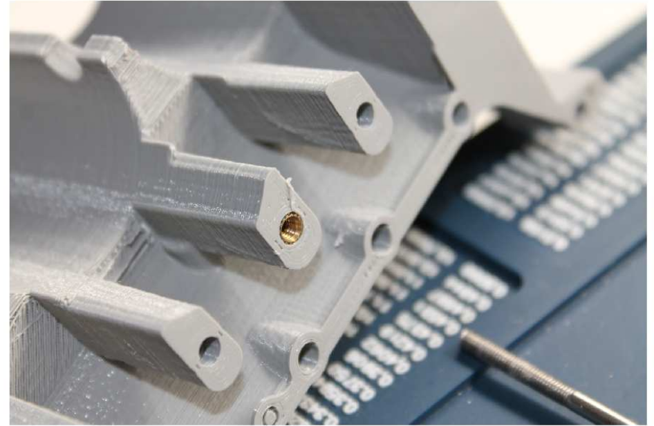
Threaded insert should be flush with surface.
