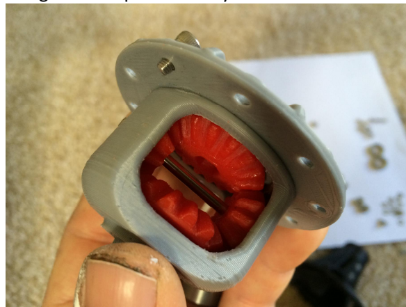
Install the two smaller spider gears and pin. You may need to remove the ring gear to install the pin.
