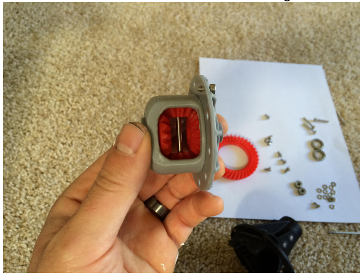
Install the two smaller spider gears and pin. You may need to remove the ring gear to install the pin.
