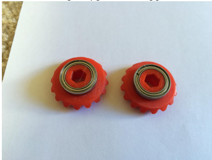
Install the two 623zz bearings onto the spider gears.
