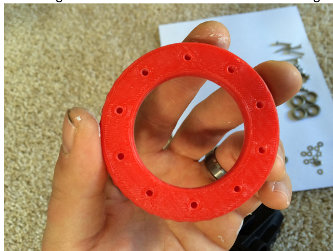
Clean and tap all the holes in the ring gear.
