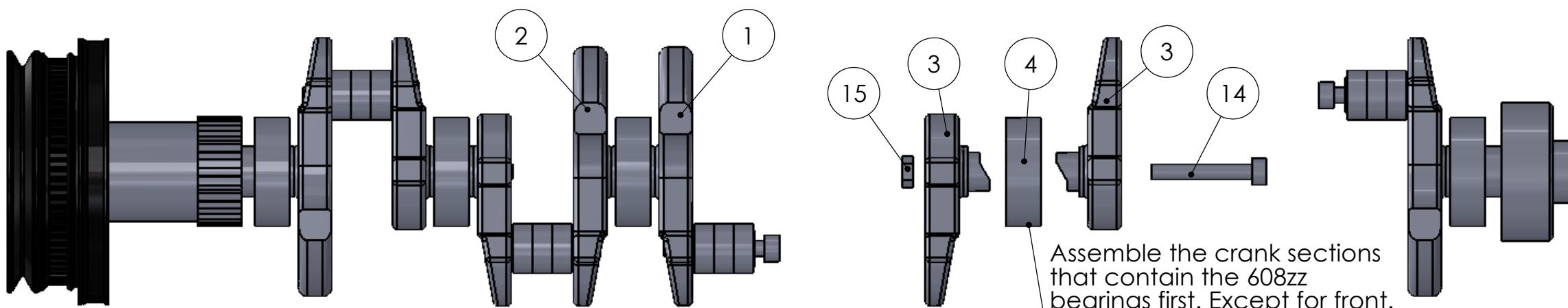
Assemble the crank sections that contain the 608zz bearings first. Except for front. Then assemble the rest.
