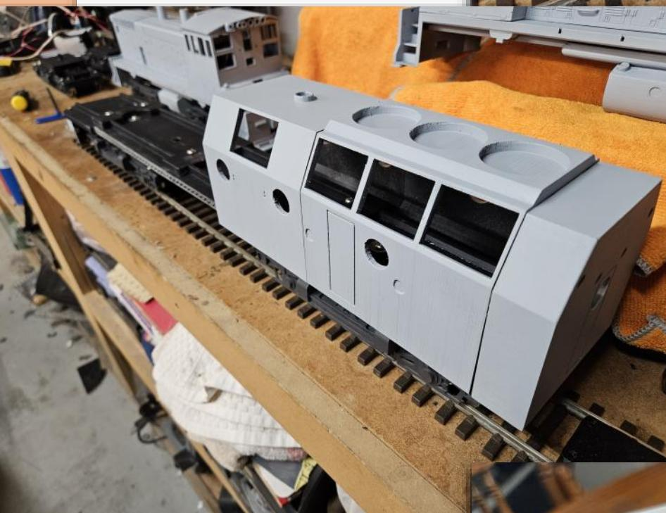
I use grey automotive primer to paint the body panels. This will give the paint a good surface to adhere to when I reach that step.
