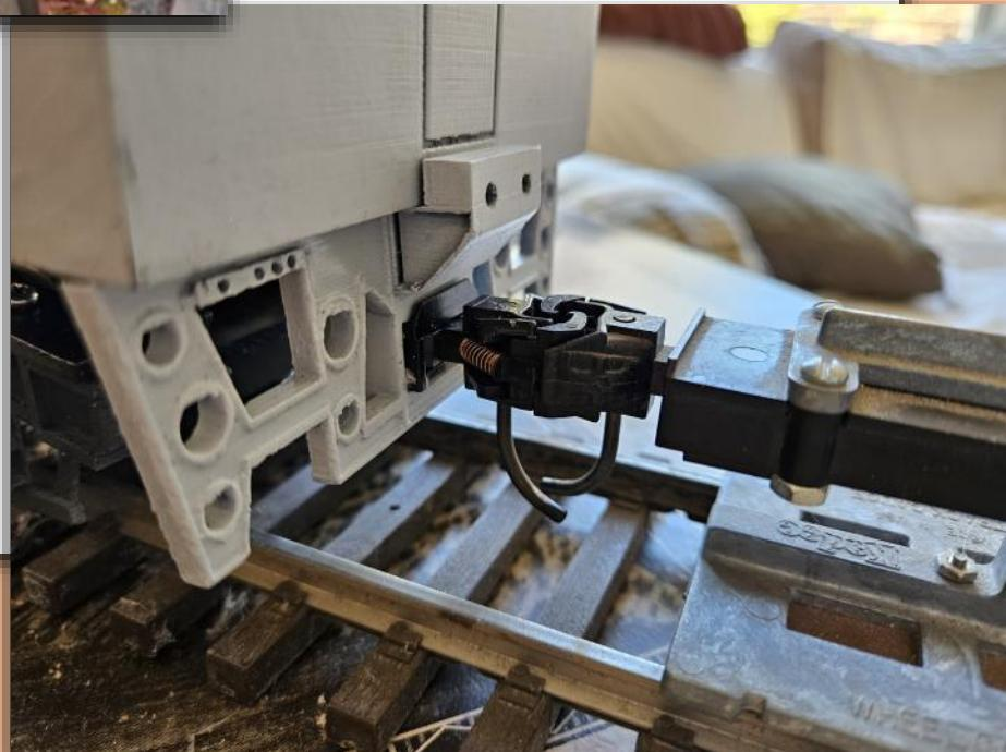
Now that I had a complete body and fuel tank, along with a working set of couplers, I decided that it was time for a “road test.” I added a temporary AirWire receiver and Li-ion battery pack and ran the locomotive in order to check mechanical function and clearances. I hooked up my “tourist train” and set off around the layout to spot any problems. I was pleased to see that the locomotive negotiated every single curve and turnout on my layout without any problems.
