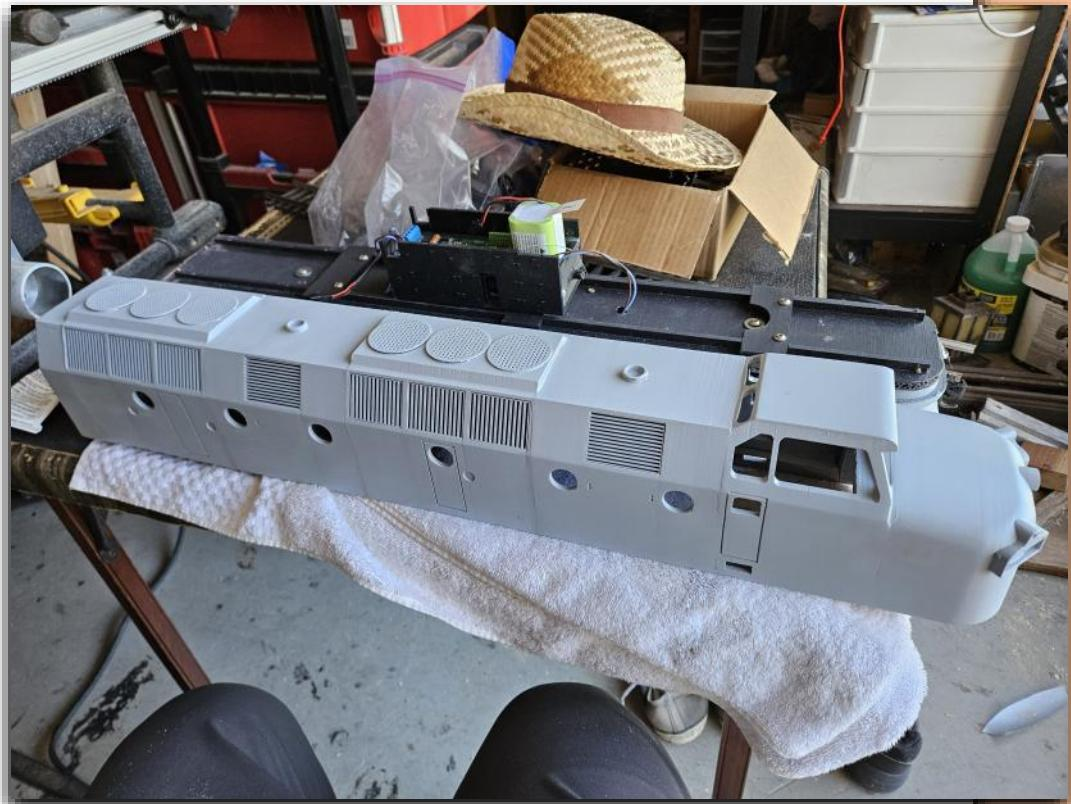
The fuel tank provides some structural rigidity to the base to keep it from flexing. I decided to make the fuel tank hollow in order to provide the option to add weight to it. After running some tests on the track, I decided to add one pound of lead weight to the bottom of the fuel tank.
