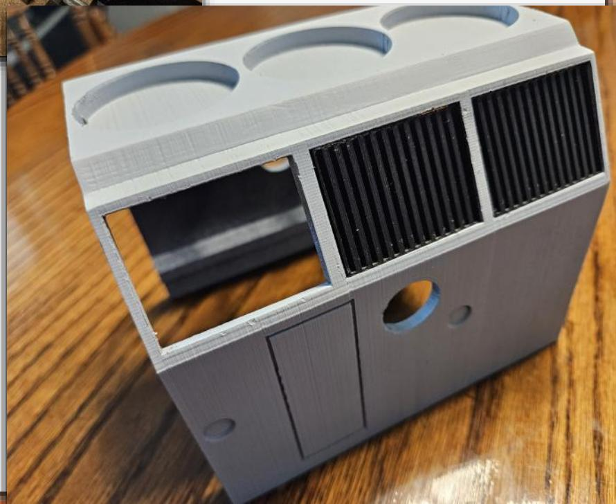
The cab took about 30 hours to print. I realized later that I needed to redesign the overhang over the windshield, which is supposed to be rounded off. I eventually rounded it using a file and auto body filler on my prototype, but the rounded overhang is now part of the design and the next one printed will be correct.
