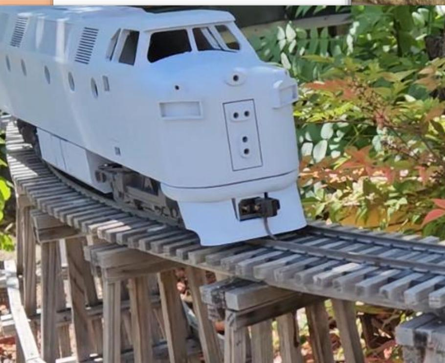
challenging. I studied the very few photos that I could find of the rear of the KM, and designed a support structure for the rear Kadee coupler. After three print and design iterations, I was able to produce a coupler mount that worked.
