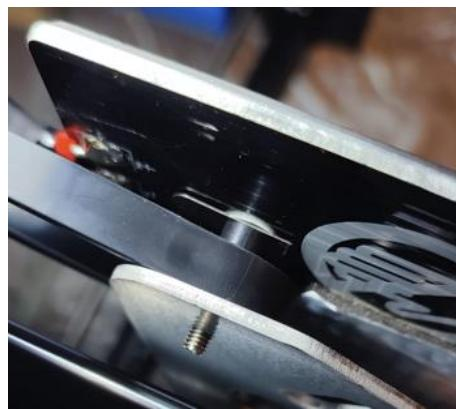
After all the shims are fitted, nip up all of the screws (**Do not fully tighten**), put the build plate back on.
