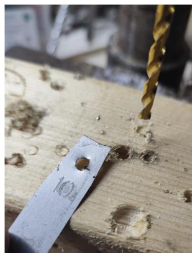
ii) Cut the hole out of the feeler gauge to make the shim, I found the best tool was my multi tool grinder
