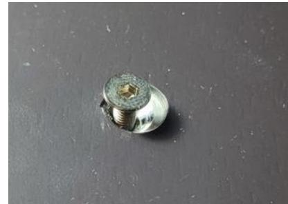
iv) Add the shims and washers to each corner in turn, remove the screw and slide the shim in. I found tweezers very helpful.
