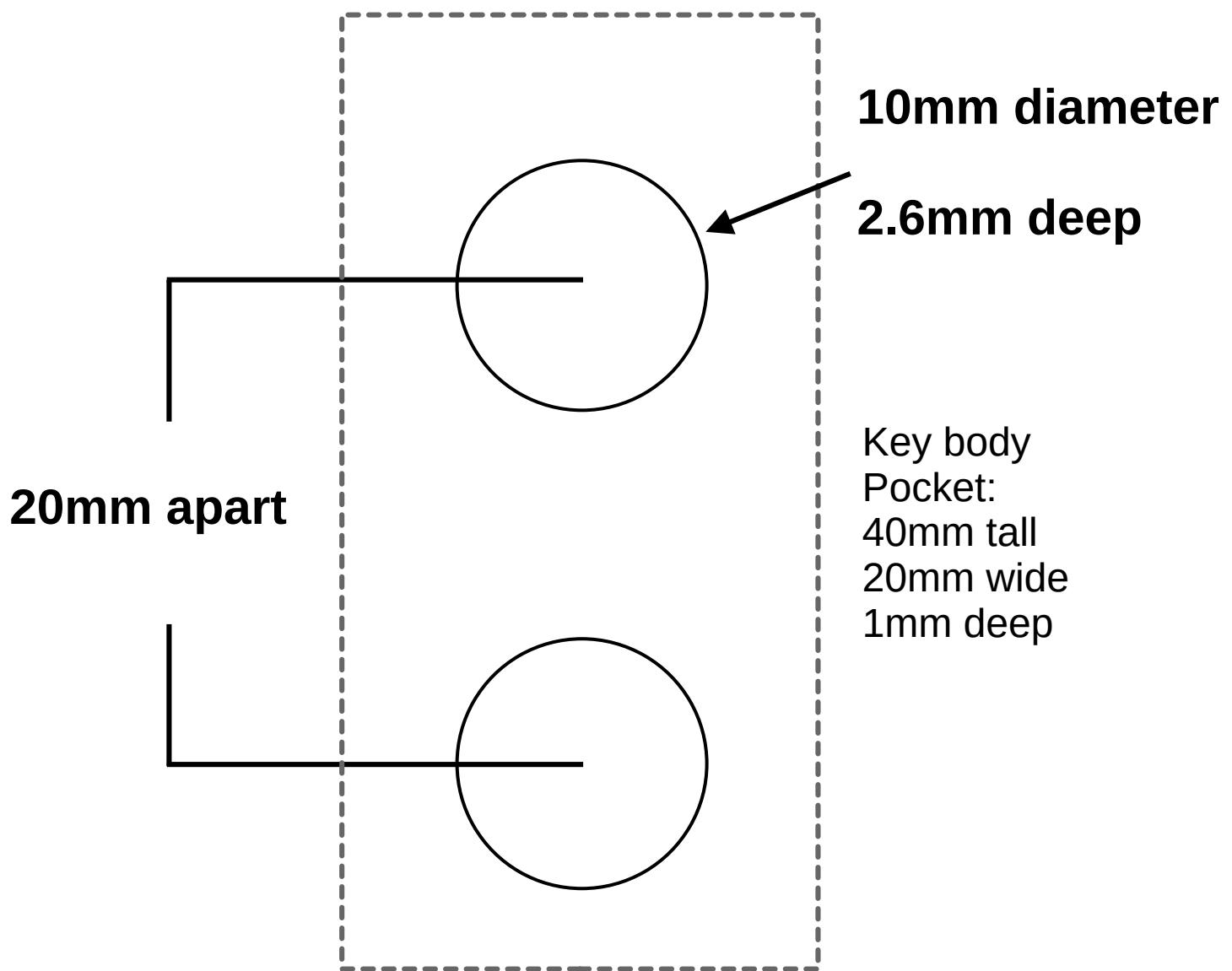
If modeling your own special mount, create two pockets for the magnets using the above dimensions.
