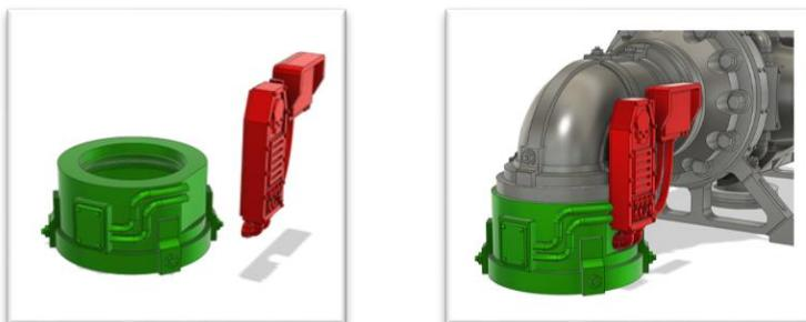
The spacer has a flat surface at the side where the Bit\_1 can be placed. The Spacer lifts the Wellhead or the 90d pipeline up to the Pipe connection on the Reactor
