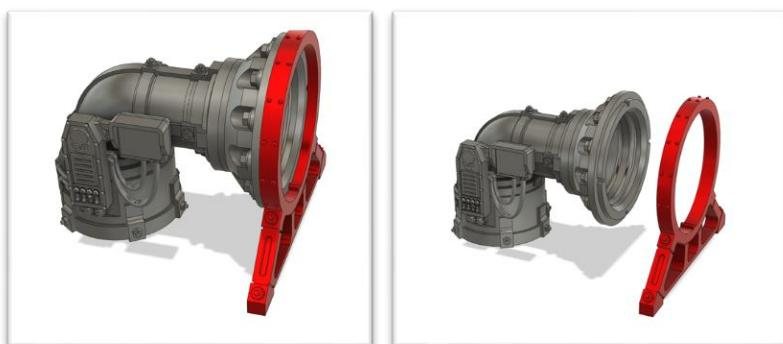
The Stand\_40mm can be printed flat on the printbed. It is designed to lift the reactor to a center height of 30,5mm. There is a little nub at the bottom that helps to align the connector\_ring at the correct angle.
