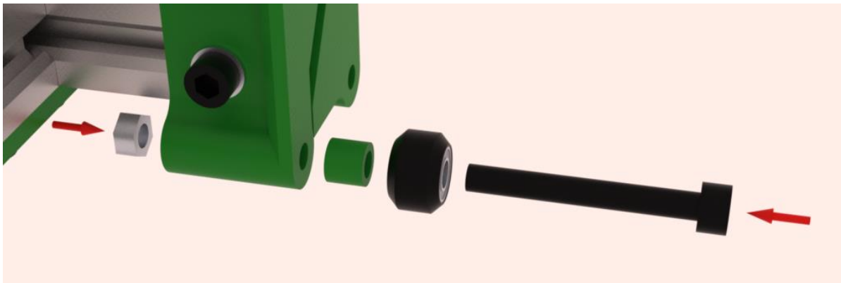
Figure 22: Z Wheel Assembly
