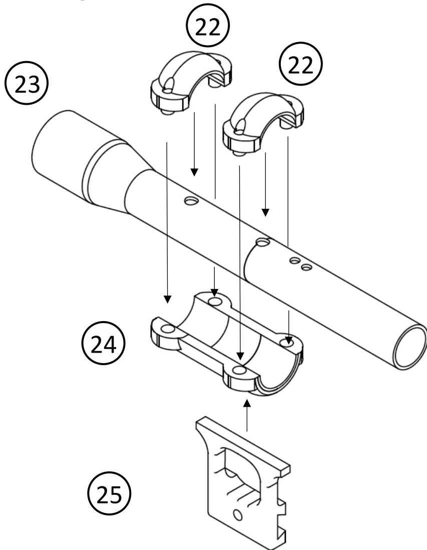
Note: Superglue is recommended secure fit between Part 24 and Part 25.
