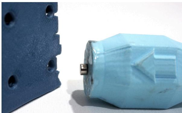
If you find some holes are too tight to press in the magnets, you may want to take a 5 mm drill bit and just loosen it a bit using your hands. The holes on the bottom of the floor pieces are more likely to be tight than the pillar and crossbeam pieces.
