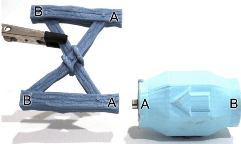
When putting magnets into the floor, the arrow should point towards the floor as you install them.
