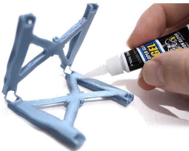
Use a Q-tip or tissue dipped in isopropyl alcohol to clean up any super glue that squeezes out of the cracks.
